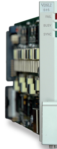
VDSL2 6+6 plug-in card with ADSL2+ and bonding.
